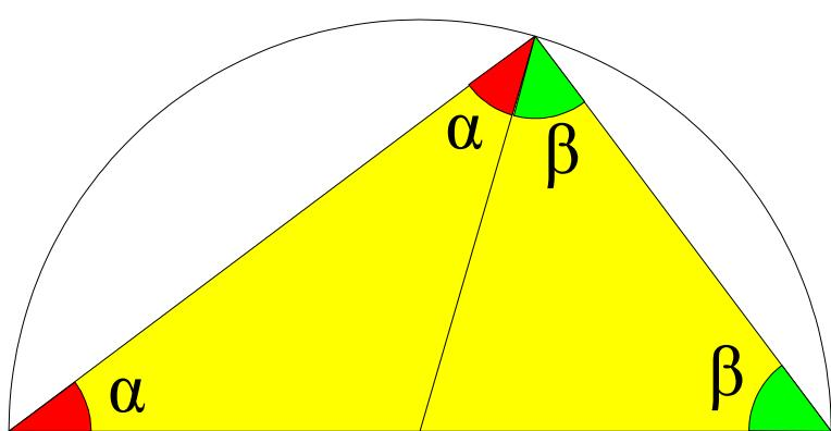
$$\begin{aligned}\alpha + \beta + (\alpha + \beta) &= 180^\circ \\ \alpha + \beta &= 90^\circ\end{aligned}$$
